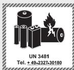
The product is equipped with or supplied with a lithium-ion battery. Do not throw the batteries into a fire and do not subject them to high temperatures. There is a risk of explosion!
