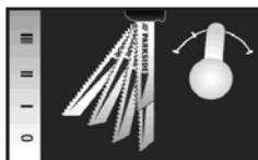
You can set the pendulum movement of the saw blade **[14]** using the pendulum action switch **[12]**. By having no pendulum action (setting "0") you can produce fine, clean cut edges. Turn off the pendulum action for thin workpieces.
