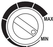
The temperature regulator ③ is steplessly adjustable. By turning it clockwise a higher temperature is set, by turning it anti-clockwise a lower temperature will be set.
