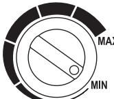
The temperature regulator ③ is steplessly adjustable. By turning it clockwise a higher temperature is set, by turning it anti-clockwise a lower temperature will be set.
