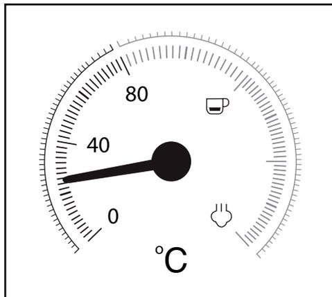
As soon as you switch the appliance on, it starts heating up until the pointer is approximately in the middle between 80°C and “☕”.
