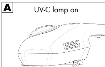
If the safety switches lose contact with the substrate, the automatic switch-off function is activated and the UV-C lamp **8** stops lighting (figs. B and C).
