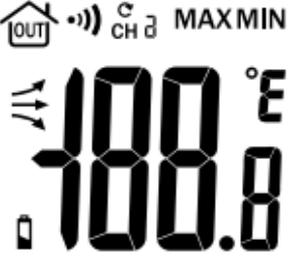
The outdoor temperature is displayed to one decimal place. The temperature unit °C (degrees Celsius) is shown top right. The temperature unit can also be changed to °F (degrees Fahrenheit).
