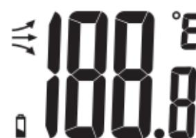
The indoor temperature measured by the temperature station is displayed to one decimal place. The temperature unit  $^{\circ}\text{C}$  (degrees Celsius) is shown top right. The temperature unit can also be changed to  $^{\circ}\text{F}$  (degrees Fahrenheit).
